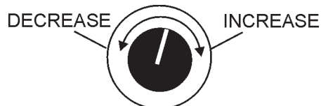
Figure 9. Voltage Regulator Control Knob
